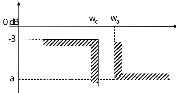
Using the expression of the Frequency response above, compute the minimal order of the filter that respects the constraints (as a function of the parameters  $w_c, w_a$  et  $a$ )
